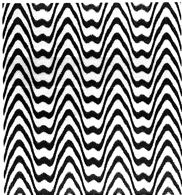
Fig. 2. Profile of a DIPEPA acrylate film after 4 min of irradiation at room temperature and \lambda = 50 \mu\text{m} .
